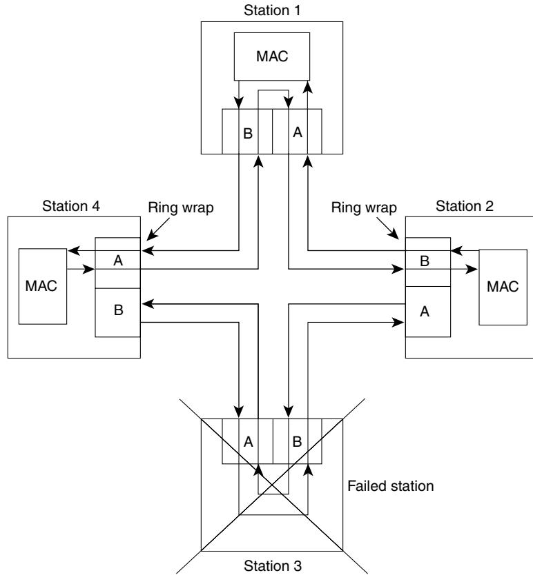
**Figure 8-7 A Ring also Wraps to Withstand a Cable Failure**
